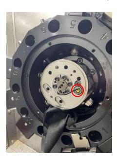
4. 檢查刀塔端及動力刀座耦合齒是否受損,動力刀座安裝前是否有做定位確認 Check whether the couplings at turret side and live tool holder side are intact without damage. Positioning of live tool holder must be done before mounting to the tool disc.
