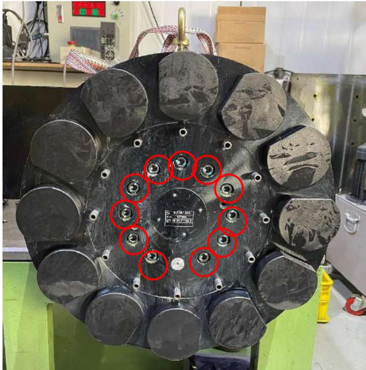
M8 螺絲扭力為 41Nm \ M8 torque is 41Nm
