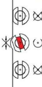
Tool drive not in zero - position. Rotating or indexing is not possible.
