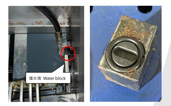
the turret. Replace with a new O-ring when necessary.
