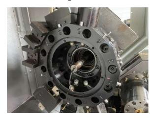
齒輪頭拆除後,請在一號刀位將刀盤固定螺絲取下,使用膠槌敲擊刀盤背面取刀盤,(拆卸刀盤請使用吊具固定刀盤,以免人員受傷),移除刀盤時注意油壓芯軸不要撞擊到。 After removing the gearhead, unfasten the fixing screws of the tool disc at T1 station. Use a plastic hammer to tap the rear side of the tool disc to take it out. Use hooks on top of the tool disc and lift it up with a crane to avoid any danger. When disassembling the tool disc, ensure not to damage the hydraulic shaft.
