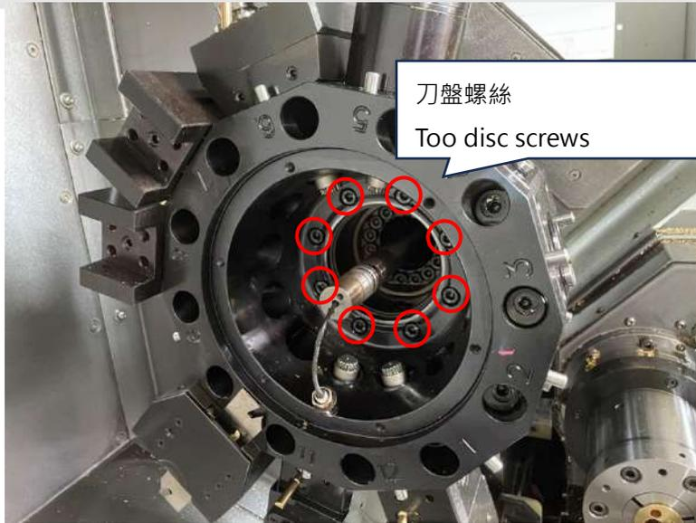
M8 螺絲扭力 39Nm \ M8 screw torque 39Nm
