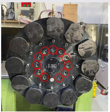
M8 螺絲扭力為 41Nm\ M8 screw torque is 41Nm
